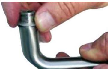
**5** After detaching the escutcheon plate, remove the nylon washer sleeve from the handle and save.
