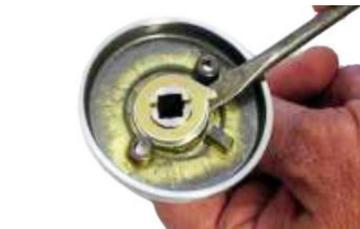
**4** Remove the stop washer and the additional washer.
