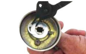
**2** Remove the snap ring and washer underneath.
