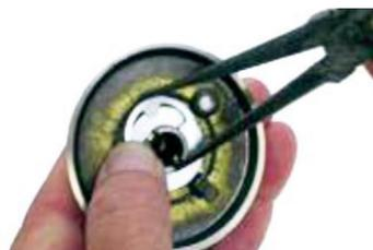
**11** Reinstall the snap ring. If it doesn't fit, you may need to remove a washer.
